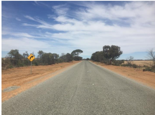
Boodarockin Rd at SLK 16.89 B – showing warning curve sign in advance of end T.P. of LH curve section from SLK 16.40 to 16.68.
