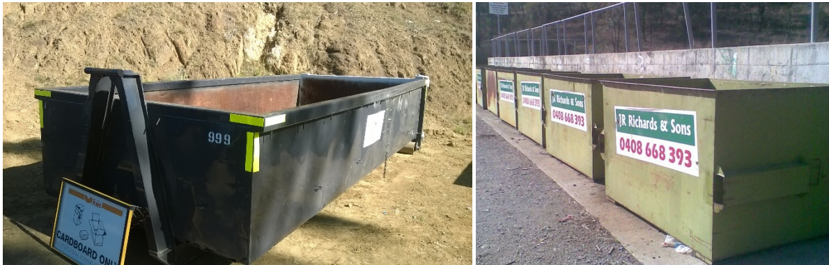
Figure 4.2 Example of hook-lift bins and front lift bins used at transfer stations
